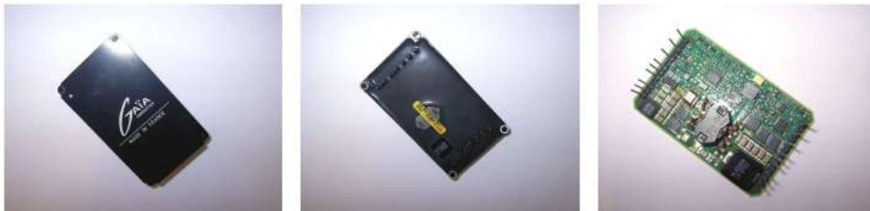
GAIA CONVERTER demonstrator (High reliability power converter)
