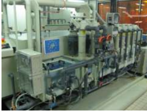
Equipment for Ni/Au finish cleaning located at SGCI (subsidiary of CIRE)
