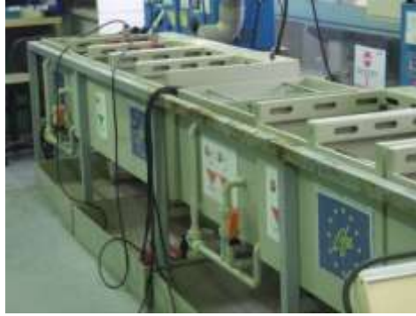
Electrolytic plating process line implemented at TEMEX CERAMICS
